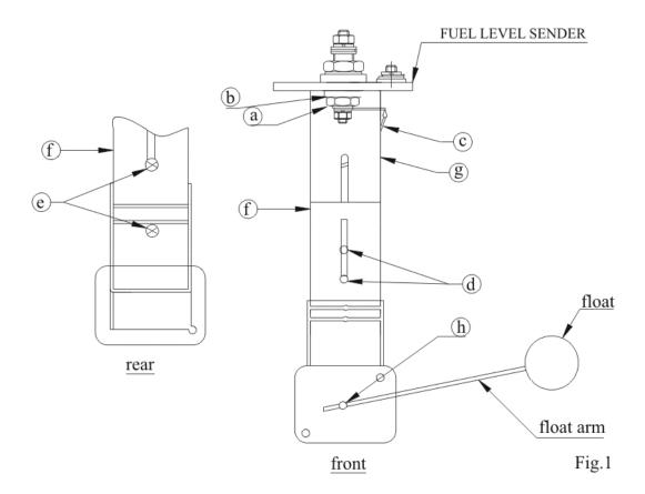
**III.** For tank depths of 16" to 21" no disassembly of the sender bracket is necessary.
