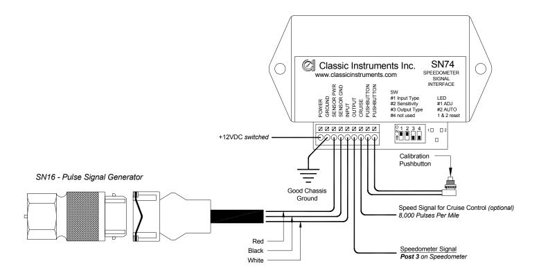
SN74 Connected to a SN16 Pulse Signal Generator
