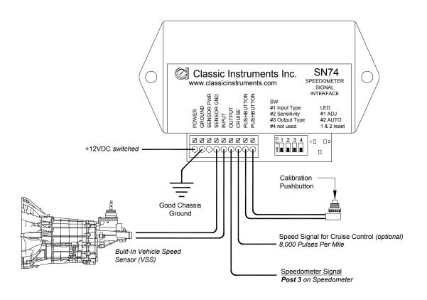
SN74 Connected to Vehicle Speed Sensor (VSS)
