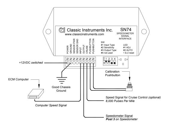
SN74 Connected to ECM Speed Signal
